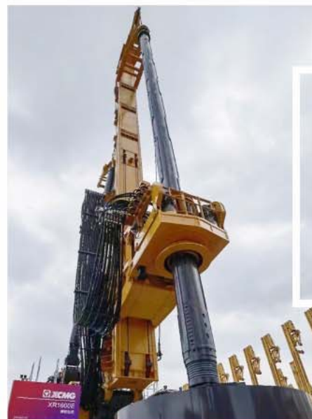
Model: OD930 -5×25m/Interlocking Max Drilling Depth: 115m
